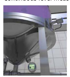
To measure continuous level of liquid in the tank, Baumer offers a variety of sensors for all needs. With hydrostatic technology the PLC will receive constant level information even under extreme temperature conditions up to 200 °C in permanent operation.
