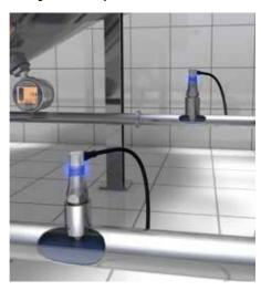
The level switch protects the pump from running dry during filling and emptying of the tank or pipe. Especially in processes where foam can occur the sensor must decide if the media is just foam or liquid. Conventional sensors have problems detecting these conditions.
